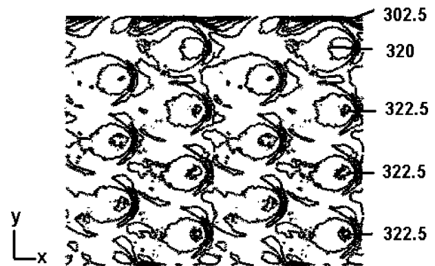
Fig. 15. Temperature contours on rotor for case with heat generation due to solid contact friction and heat conductive bristle tops (contour interval = 2.5 K).
